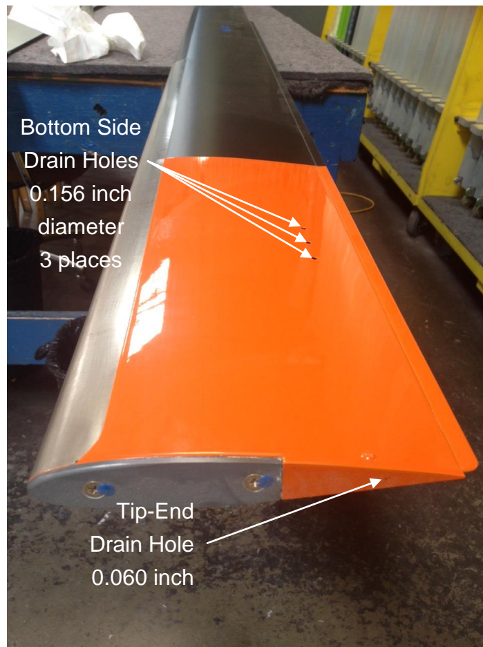
Figure 5 – Tip of Main Rotor Blade - Drain Holes (Bottom Side Shown)
